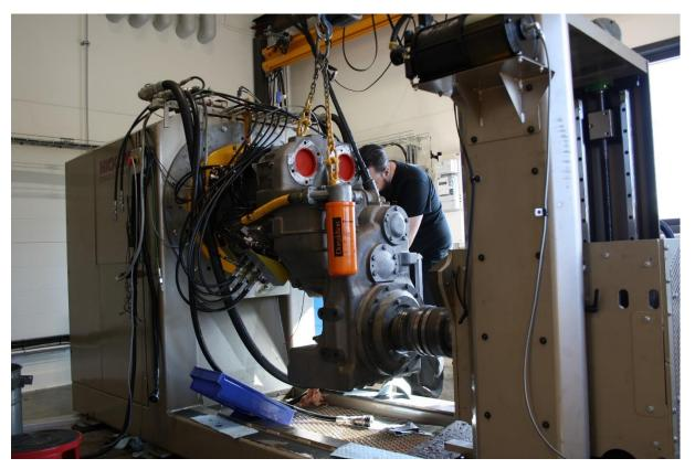
Simulating where the pressure of each gear is checked in-line with factory specifications.
